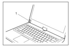
➤ You must install the fingerprint software in order to be able to use the fingerprint sensor (1).
